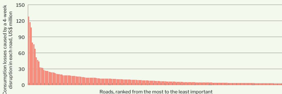
Benefits from strengthening different road segments in Tanzania considering their criticality
